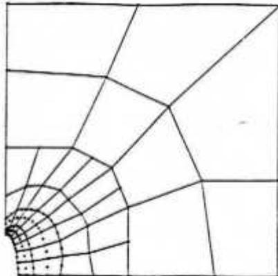
Figure 7. Improved Mesh (40 Elements, 113 Nodes, 3r-p-1r-hp-1r Trajectory)
