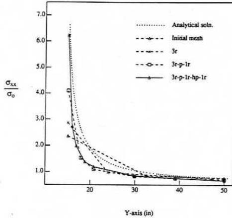
Figure 10.  $\sigma_{xx}/\sigma_0$  Along the Y-axis (36 Elements, 136 Nodes), 1 in = 25.4 mm
