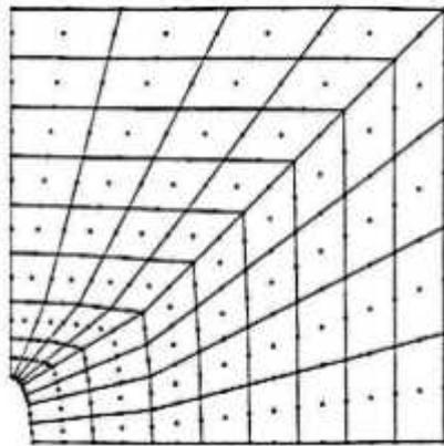
Figure 11. Improved Mesh in Global Refinement (64 Elements, 289 Nodes, p-hp Trajectory)
