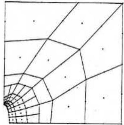
Figure 8. Improved Mesh in Semi-Global Refinement (36 Elements, 139 Nodes, 3r-p-1r-hp-1r Trajectory)
