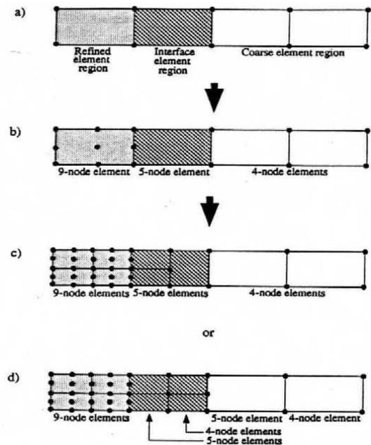
Figure 2. Regional Refinement with Collapsible Element
