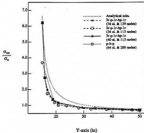
Figure 13. Comparison of  $\sigma_{xx}/\sigma_0$  Along the Y-axis for Regional and Global Improvement Cycles, 1 in = 25.4 mm
