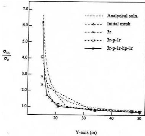
Figure 6.  $\sigma_{xx}/\sigma_0$  Along the Y-axis (36 Elements, 113 Nodes), 1 in = 25.4 mm
