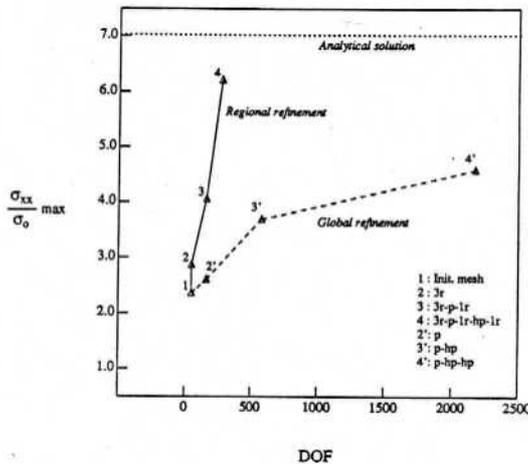
Figure 14. Comparison of Maximum  $\sigma_{xx}/\sigma_0$  in Terms of DOF Used in the Regional and Global Refinements
