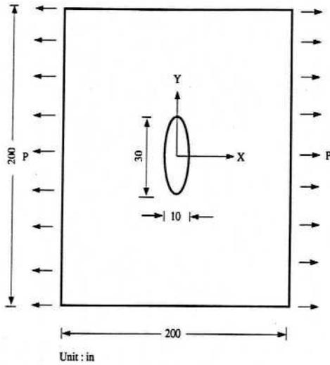
Figure 4. Square Plane, 200 × 200 in<sup>2</sup> (5080 × 5080 mm<sup>2</sup>) with an Elliptic Hole, 30 in (762 mm) - 10 in (254 mm)
