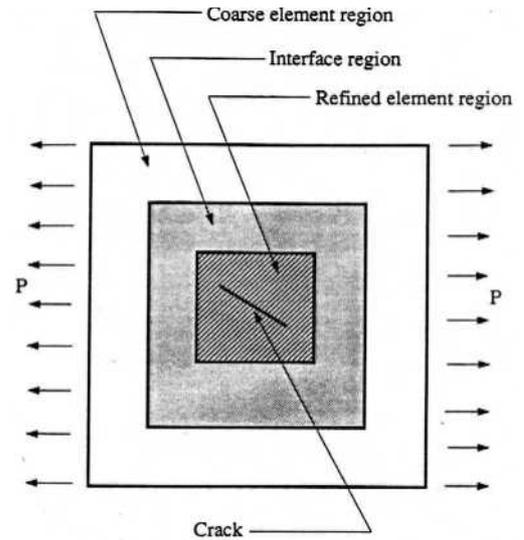
Figure 1. Regional Refinement for a Crack Problem
