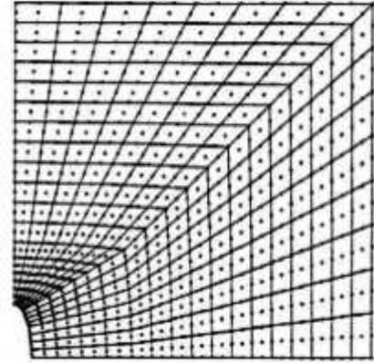
Figure 12. Improved Mesh in Global Refinement (258 Elements, 1089 Nodes, p-hp-hp Trajectory)
