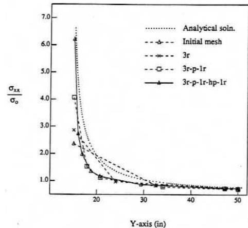
Figure 9.  $\sigma_{xx}/\sigma_0$  Along the Y-axis (40 Elements, 113 Nodes), 1 in = 25.4 mm
